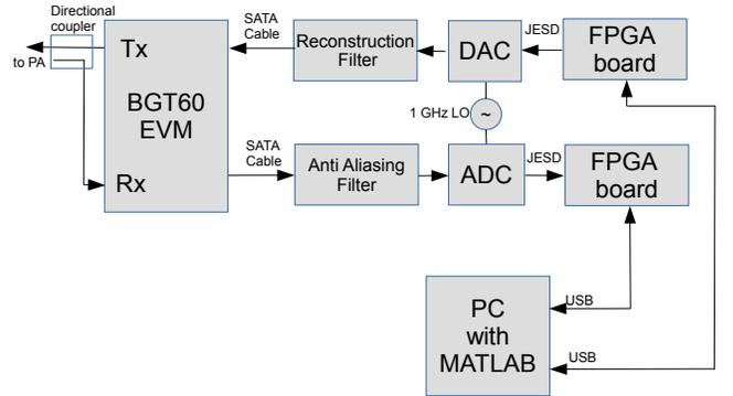
Fig. 2: Block schematic of the 60 GHz setup used for RF front-end parameters extraction [4]
