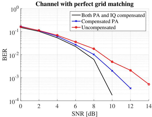
Fig. 5: Bit error rate, RF impairments and channel with perfect grid match
