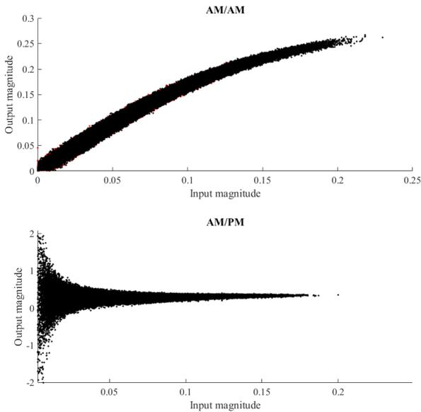
Fig. 3: Extracted AM/AM and AM/PM characteristics of 60GHz power amplifier
