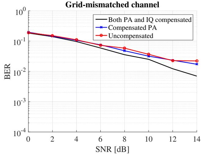
Fig. 6: Bit error rate, RF impairments and channel with grid mismatch of 20%
