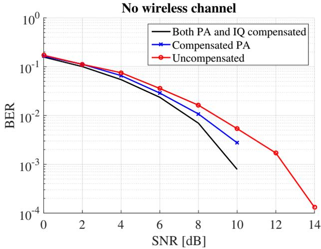
Fig. 4: Bit error rate, without channel, only RF impairments
