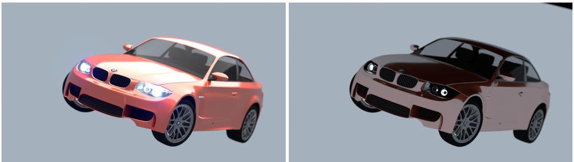
Figure 5.9: The test scene “Car Demo”. The left image depicts the intended outcome as rendered by Cycles, the right image shows how it is rendered by LuxCoreRender.
