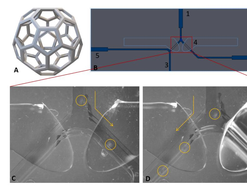
**Table: Figure 1** Automated tissue sorting system (A) 3D model of a scaffold for spheroid culture (B) CAD model of microfluidic sorting chip. Scaffolds (yellow) are either delivered to the waste channel (C) or the ejection channel (D). **Results and discussions:** Scaffolds were produced in a shape resembling a Buckminster fullerene with a diameter of 300 µm and an overall porosity of 96% to promote rapid cell invasion (Figure 1 A).
