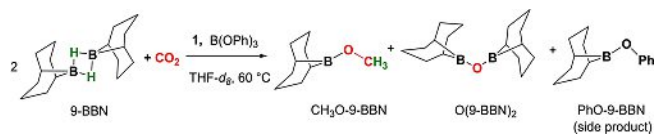
Scheme 3. CO 2 hydroboration in the presence of 1 and 9-BBN.
