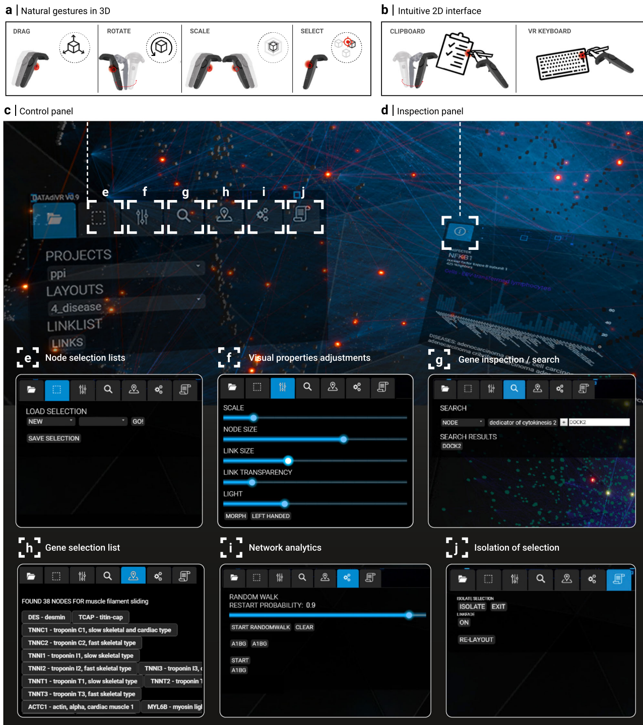
Fig. 3 User interaction design. a Interactions with the 3D network, such as moving the network or selecting individual nodes, are implemented as natural 3D gestures. The movement of the controllers with pressed trigger buttons (indicated in red) is directly translated into the corresponding movement of the network, allowing the user to drag, rotate, and scale the network. Individual nodes are selected by directly pointing at them. b , All other interactions are performed through 2D interfaces dedicated to specific tasks. The core functionalities are collected into a control panel that spawns as a virtual clipboard in one hand, and a virtual stylus in the other, which can also be used to type on a virtual keyboard. VR screenshots showing the (c) control panel and a particular (d) inspection panel. Inspection panels are used to display the results of a particular action or analysis, such as providing detailed annotations for a selected node. e–j Screenshots of the different core functionalities, organized as different tabs in the control panel. e Loading (saving) specific node sets from (to) the database. f Adjusting visual properties of the network. g Searching for nodes and node sets, either by name or any other attribute contained in the database. Searches can also be combined using logical operators. h List of currently selected nodes. i User interface for running network analytics, such as random walk with restart from a selected node set. j Highlighting node selections.
