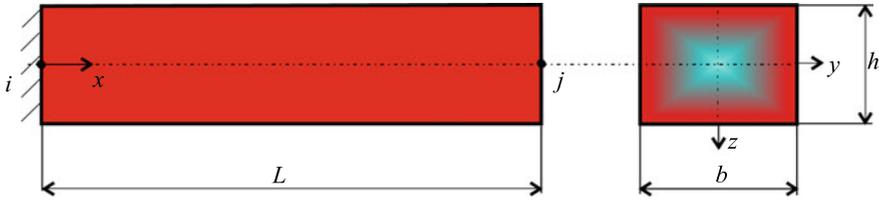
**Fig. 4** A straight FGM beam of the rectangular cross-section with the varying material properties in two directions
