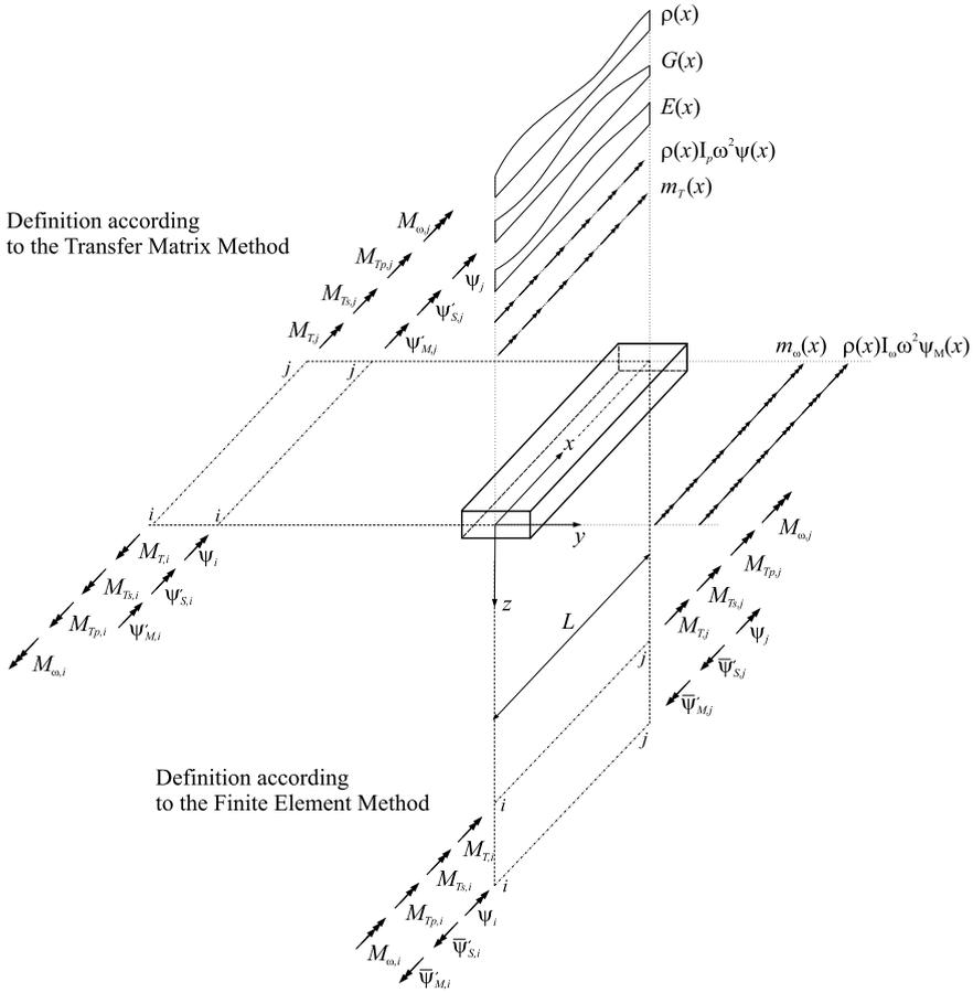
**Fig. 2** Positive orientation of the moments and rotation angles at element nodes for the TMM and the FEM
