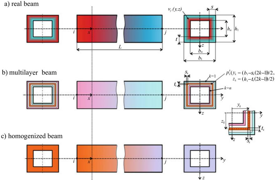
Fig. 3 A straight FGM beam of the hollow cross-section
