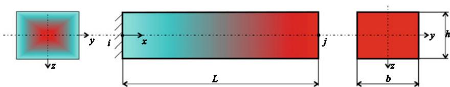
**Fig. 5** A straight FGM beam of the rectangular cross-section with the varying material properties in three directions
