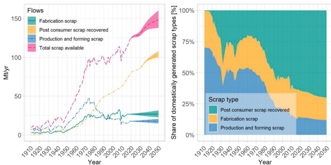
Fig. 2. left: Modelled quantities of flows scrap becoming available, categorized into forming & production scrap, fabrication scrap and post-consumer scrap as well as the total amount (sum of all scrap categories). The ribbon indicates the three scenarios (upper bound: growth; line: zero growth; lower bound: de-growth); right: Shares of scrap types: production & forming scrap, fabrication scrap and post-consumer scrap.
