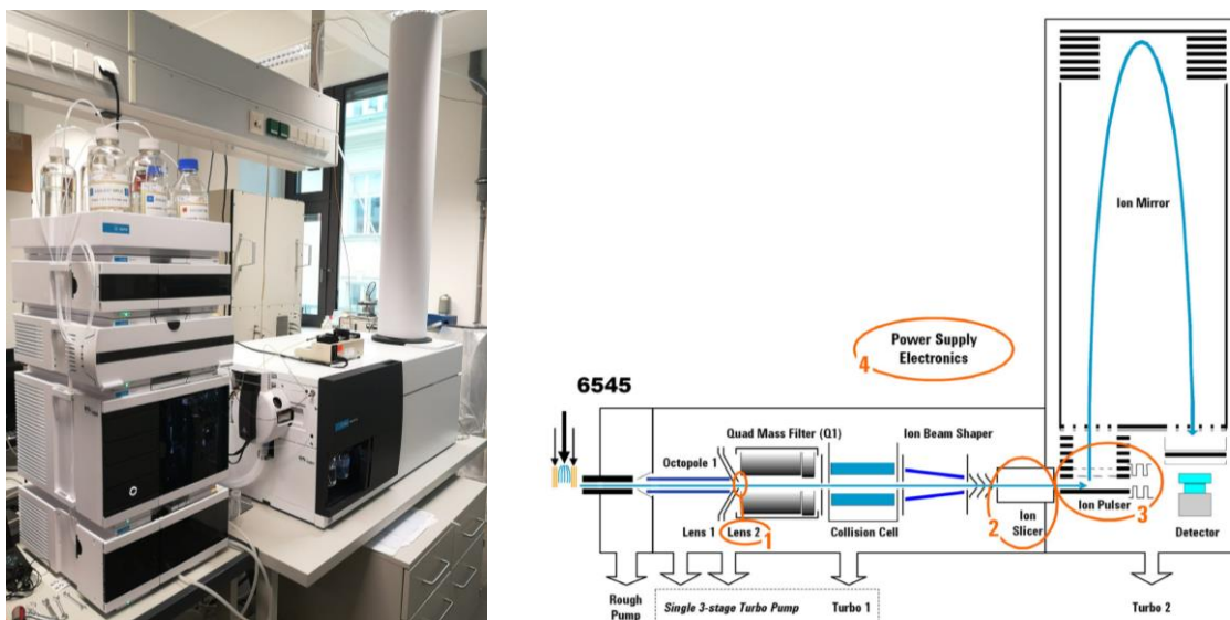
Figure 11: left: Agilent 6545 (Agilent); right: Setup of the Agilent 6545 QTOF system [32]
