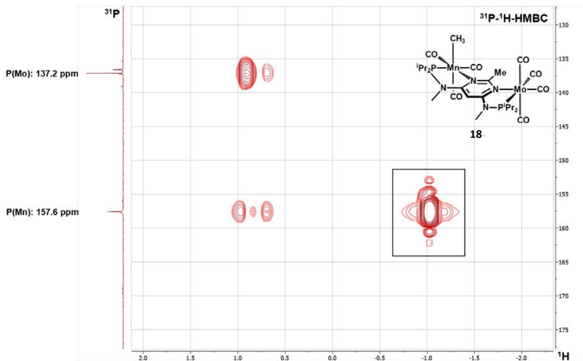
Figure 17 ^{31}\text{P}\text{-}^1\text{H}\text{-HMBC} of the reaction of 14 with \text{TINO}_3 and \text{Me}_2\text{Zn}
