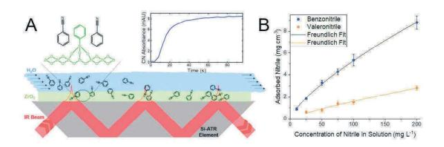
Figure 1. (A) Enrichment of an aqueous benzonitrile solution using a phenylsilylated ZrO2-coating on a Si-ATR element. (B) Freundlich adsorption isotherms for the enrichment of two analyte solutions.
