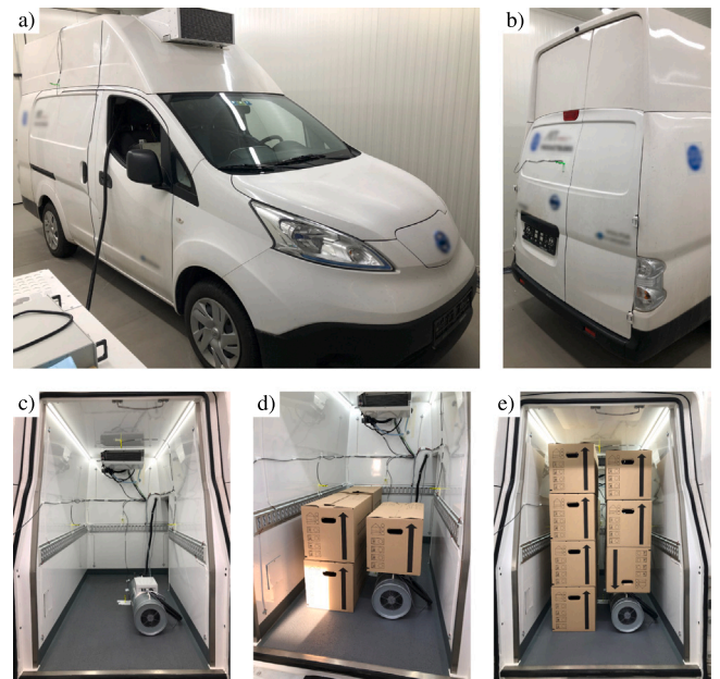
Fig. 7. Investigated refrigerated truck in (a) diagonal front view and (b) diagonal rear view. Its cooling chamber is shown in an empty, a partially filled, and a completely filled setup in (c)–(e), respectively. The fan heater, mounted on the floor of the cooling chamber and apparent from (c–e), is off throughout the whole experimental investigation within this work. Some areas of (a) and (b) are blurred for legal reasons.
