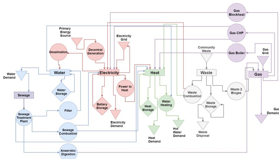
Figure A1. Gas-based energy system.
